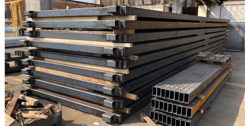
Steel pen sections before galvanization
