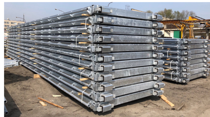
Steel pen sections after galvanization
