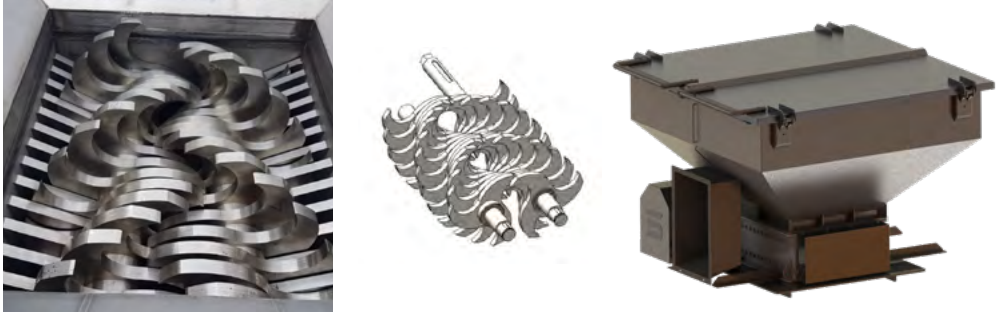
Hook-shaped blades provide maximum capacity
