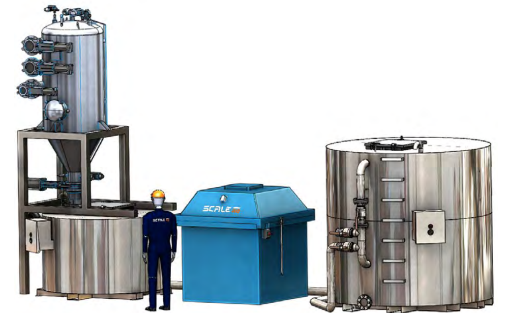
Dedicated ensilage area with a cyclone for collecting dead fish from the vacuum system, a grinding tank for fine grinding of the fish, acid dosing systems for ensilage preservation, and storage tank solutions for storing finished ensilage. All systems are customized to each facility, considering factors such as facility size, customer requirements, logistics, and more.
