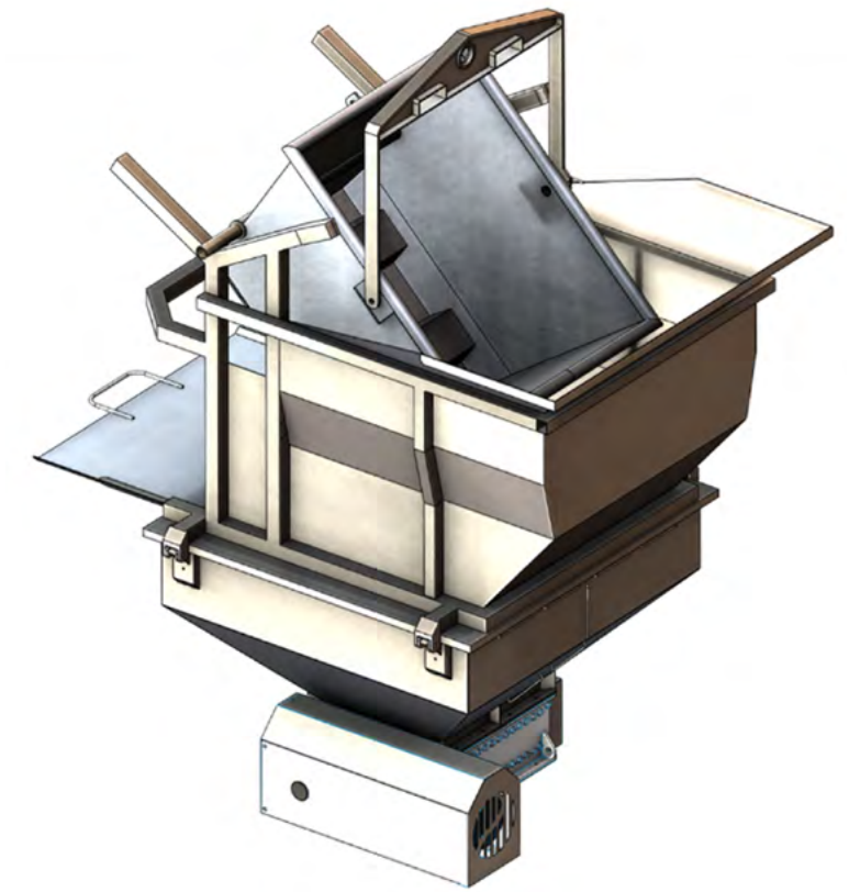
Tipping arrangement for tipping container against pre-grinders
