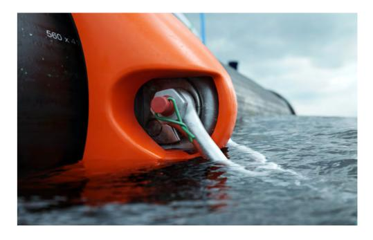
The insert is fitted to the welded mooring lug on the mooring bracket, and acts as a replaceable lining that can be worn out. The mooring lug insert can be retrofitted at sea, or supplied pre-fitted to floating collars during production. This fitting means that aquaculture operators avoid the need to replace the full mooring bracket when wear and tear exceeds the set limits.
